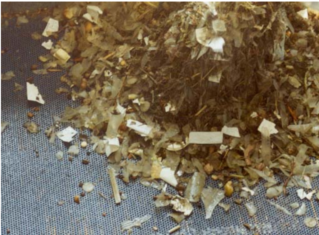
Fig. 7: Separated rough disturbing substances in the de-watering tank with a high percentage of plastic.
