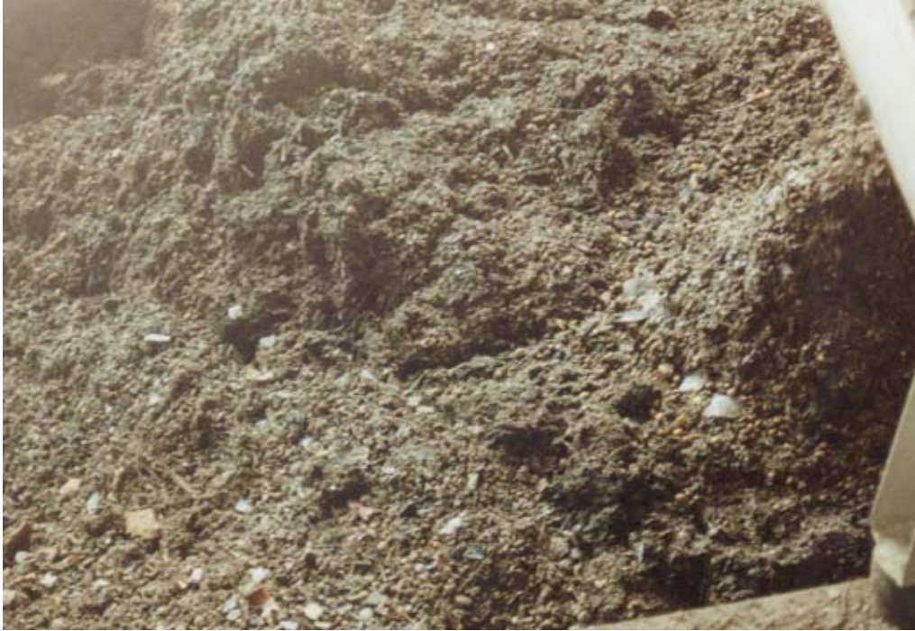
Fig. 6: Separated fine disturbing substances with a high content of sand.
