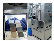
Developing efficient recycling technology for commercial laundry facilities is demanding because the quality and hygiene of laundry processes must be maintained. REWARD is overcoming this challenge by combining dipole induction technology (through pulsed high voltage) with customized membrane filtration. The process leads to high recycling rates in detergent ingredients – particularly surfactants –
