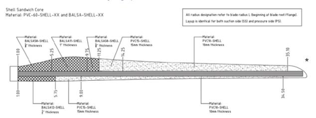
To enable drapeability of the (biaxially) curved core panels during manufacturing, foam and balsa sheets are (uni-/bidirectional) slit or knife-cut. To secure reliable vacuum infusion processing, additional perforation and grooving can be applied in specific areas. All of these cavities will be filled with resin during infusion.
